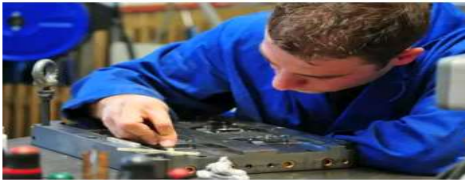
Fig2 Manual Mold Cleaning
